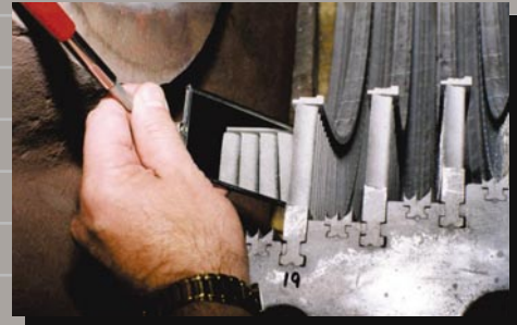
Structural and thermodynamic steampath audits are conducted to provide owners with repair recommendations accompanied by associated gains in efficiency.
