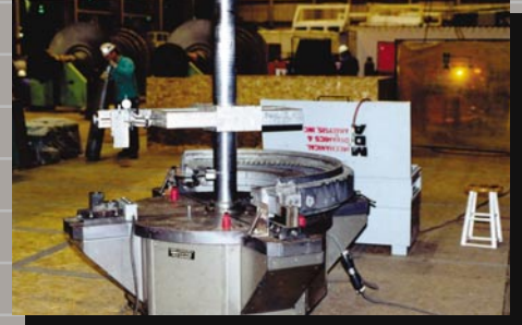
Our unique portable vertical turning lathes enable our technicians to machine blade ring and diaphragm critical fit areas on-site, eliminating shipping and promoting timely turnaround.
