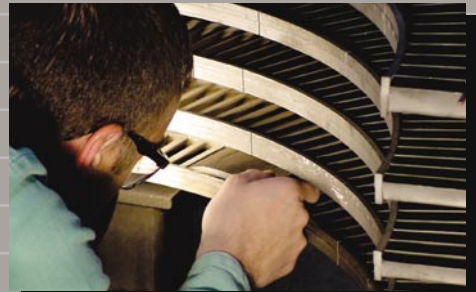
Partition & blade profiles are restored to OEM specifications and then polished to meet or exceed the original OEM specifications for surface roughness.
