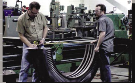
Caulked-in steam seals are replaced and out-of-roundness checked on all diaphragms and blade rings prior to final quality control checks and shipping.
