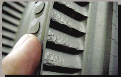
Damage caused by foreign objects is identified and repairs are recommended that can correct profiles and reduce future performance losses.
