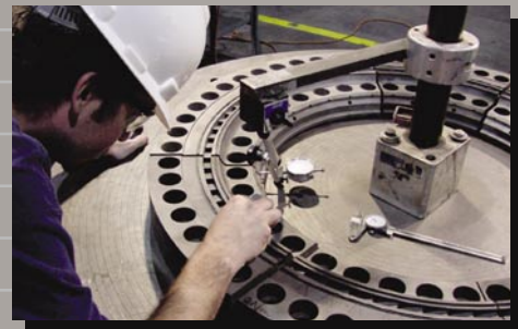
In-process and final inspections using precision instruments to assure repair quality, unit performance and reliability.
