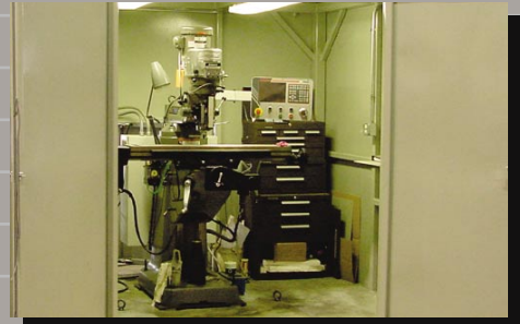
Fully CNC capable milling machines are contained in portable shipping containers for immediate transport and on-site fabrication of components such as blade shrouds and bucket covers.
